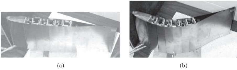
Figure 3.1. SMA multiactuated hydrofoil prototype (Rediniotis et al. [60]).
