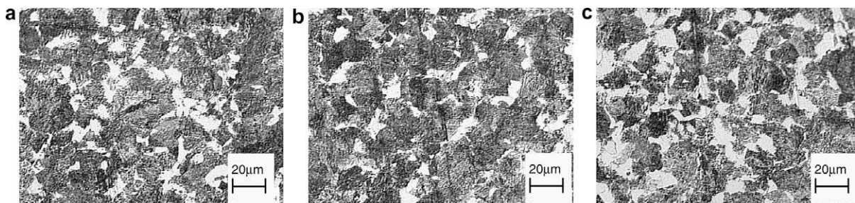
Fig. 4. Air cooling specimen microstructure: (a) center ( r = 0 ), (b) r = 0.50R and (c) surface ( r = R ). Etching nital 2%.
