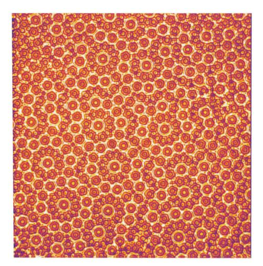
FIG. 1. (Color) A quasicrystalline wave pattern with 12-fold rotational symmetry. This standing-wave pattern was produced by forcing a layer of silicone oil simultaneously at two frequencies, using a method invented by Edwards and Fauve. The brightest regions are locally horizontal, whereas darker colors indicate inclined regions. From work done at Haverford for an undergraduate thesis by B. Pier.
